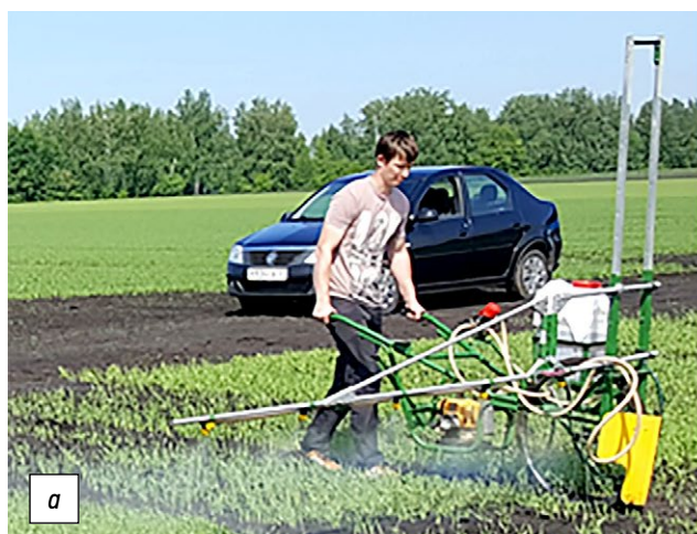
Fig. 1. A prototype of a single-support boom motor sprayer (a) and a device for measuring values of horizontal inclinations of a field boom (b).
