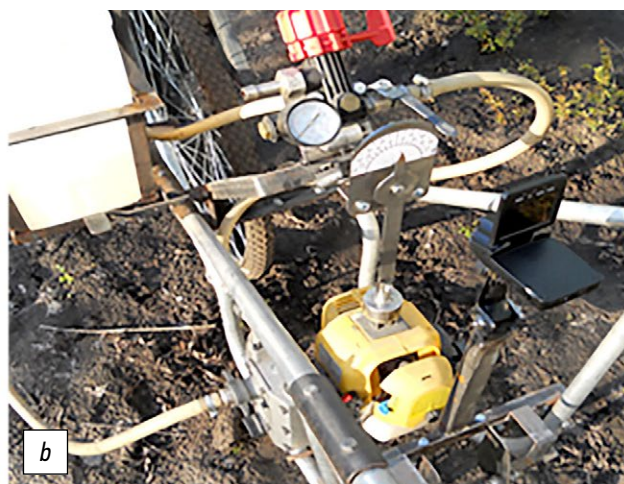
Fig. 1. A prototype of a single-support boom motor sprayer (a) and a device for measuring values of horizontal inclinations of a field boom (b).
