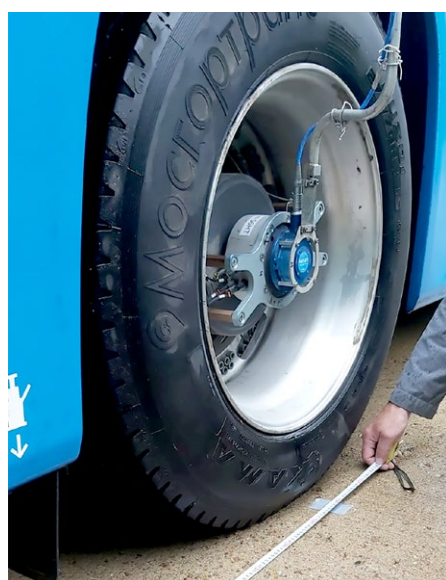
Fig. 1. Kistler–Rim RoadDyn strain gauge wheels.
