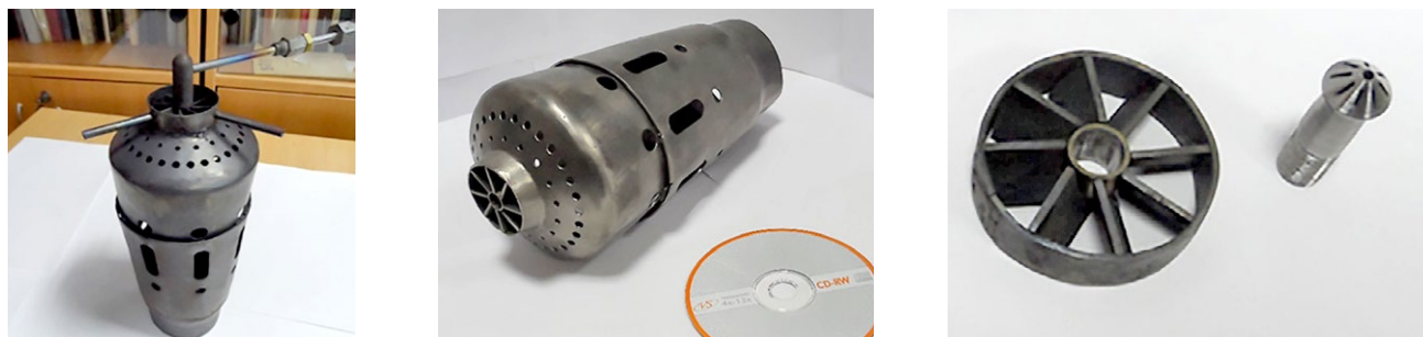
Fig. 3. The flame tube with an injector and a swirler of the individual tubular combustion chamber.
