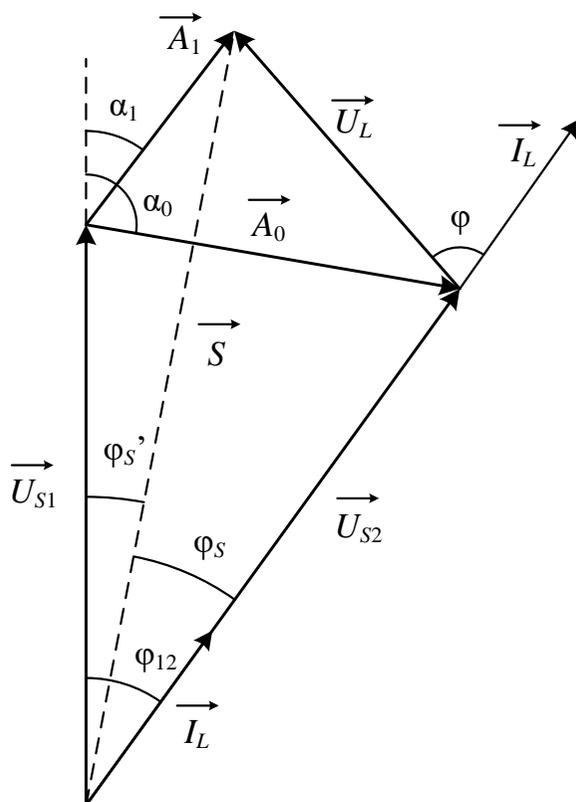
Fig. 2. Vector diagram of the current and voltage with regulation of the current parameters of the power transmission line
