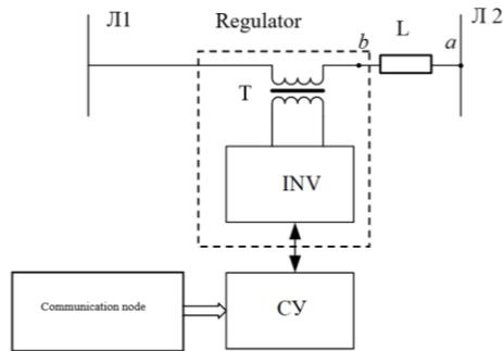
Fig. 1. Area of the electric grid with regulator installed on the transmission line
