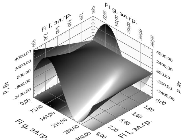
Fig. 6. Active power generated/consumed by the voltage inverter INV with leading voltage for line L2
