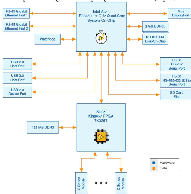
Fig. 3. Structure of platform *cRIO*
