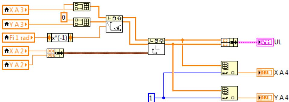
Fig. 5. Graphic of the code of the network throttle voltage vector calculation node
