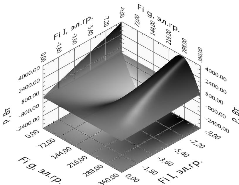
Fig. 7. Active power generated/consumed by the voltage inverter INV with lagging voltage for line L2
