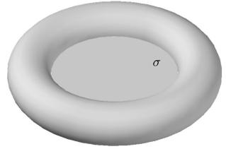
[The location of the sonic surface on the circular part of the plane of symmetry of the torus satisfies the first geometric condition]
