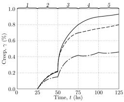
[Figure 5. Creep curves (torsion angle) of samples made of 3KhV4SF steel under step tension with torsion:  $1-\sigma=200$  MPa,  $\tau=0$  MPa;  $2-\sigma=200$  MPa,  $\tau=78$  MPa;  $3-\sigma=200$  MPa,  $\tau=115$  MPa;  $4-\sigma=136$  MPa,  $\tau=115$  MPa;  $5-\sigma=0$  MPa,  $\tau=115$  MPa; solid line — experimental data; dash dotted line — calculation assuming similarity of deviators (1); dashed line — calculation according to the proposed model
