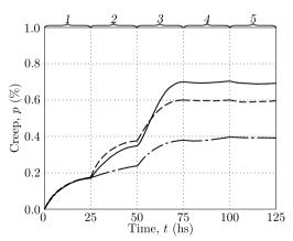
[Figure 4. Creep curves (axial deformation) of samples made of 3KhV4SF steel under step tension with torsion:  $1-\sigma=200$  MPa,  $\tau=0$  MPa;  $2-\sigma=200$  MPa,  $\tau=78$  MPa;  $3-\sigma=200$  MPa,  $\tau=115$  MPa;  $4-\sigma=136$  MPa,  $\tau=115$  MPa;  $5-\sigma=0$  MPa,  $\tau=115$  MPa; solid line — experimental data; dash dotted line — calculation assuming similarity of deviators (1); dashed line — calculation according to the proposed model
