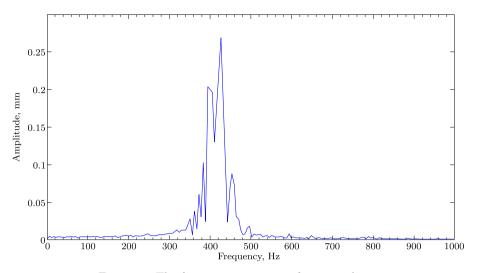
Figure 6. The frequency spectrum after smoothing
