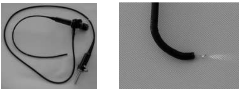
Fig. 3, 4 Flexible endoscope with laser waveguide
