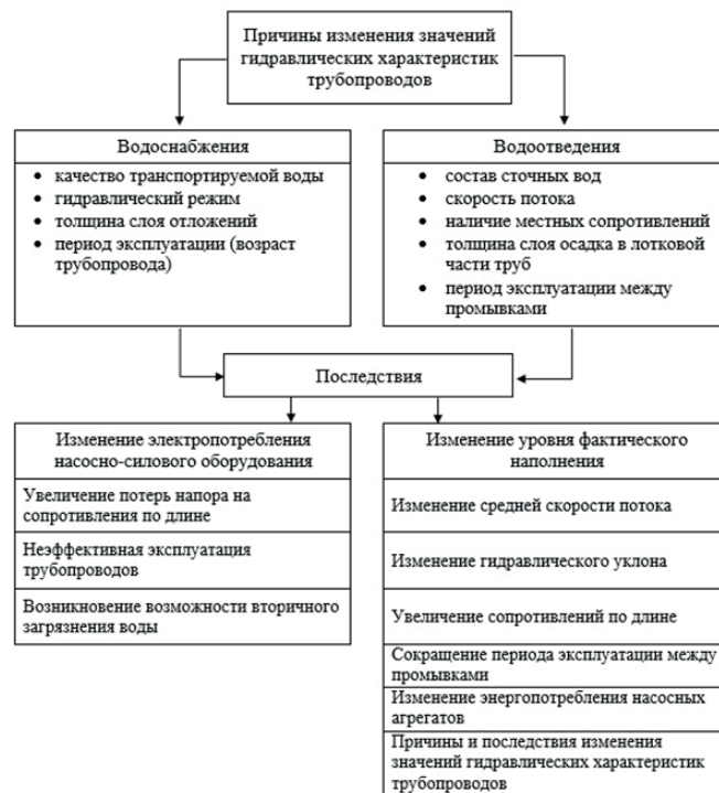
Fig. 2. Causes and consequences of changes in the hydraulic characteristics of water supply and wastewater pipelines
