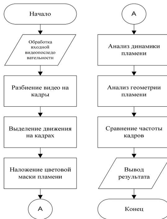
Fig. 4. Flow chart of the flame detection algorithm via video data
