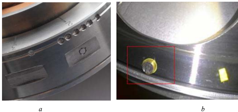
Fig. 1. Balancing the rotor-flywheel: a – removing the metal on the rim of the flywheel; b – balancing with screws
