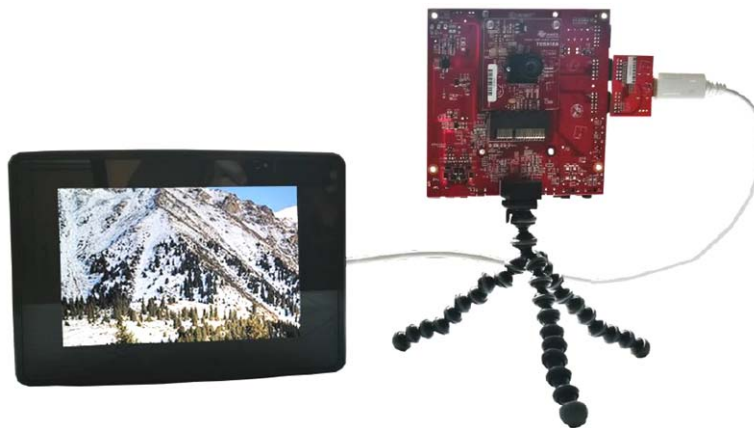
Fig. 2. Complete camera-to-touchscreen demo kit
