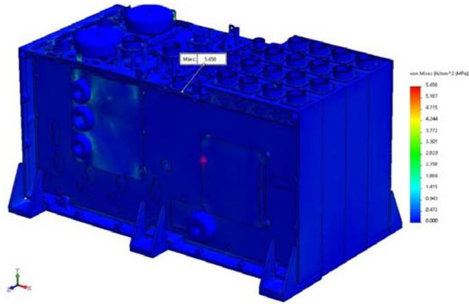
Fig. 19. Distribution of the stress in AB model at effect of random vibration along  $OY$  axis
