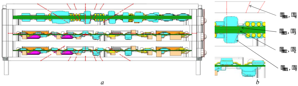
Fig. 6. Example of tracing rays passing through constructional elements of the block: a – cut-away view of the block and rays; b – line segments l_{ijk} passed by the ray in constructional elements and apparent densities of materials \rho_k corresponding to them
