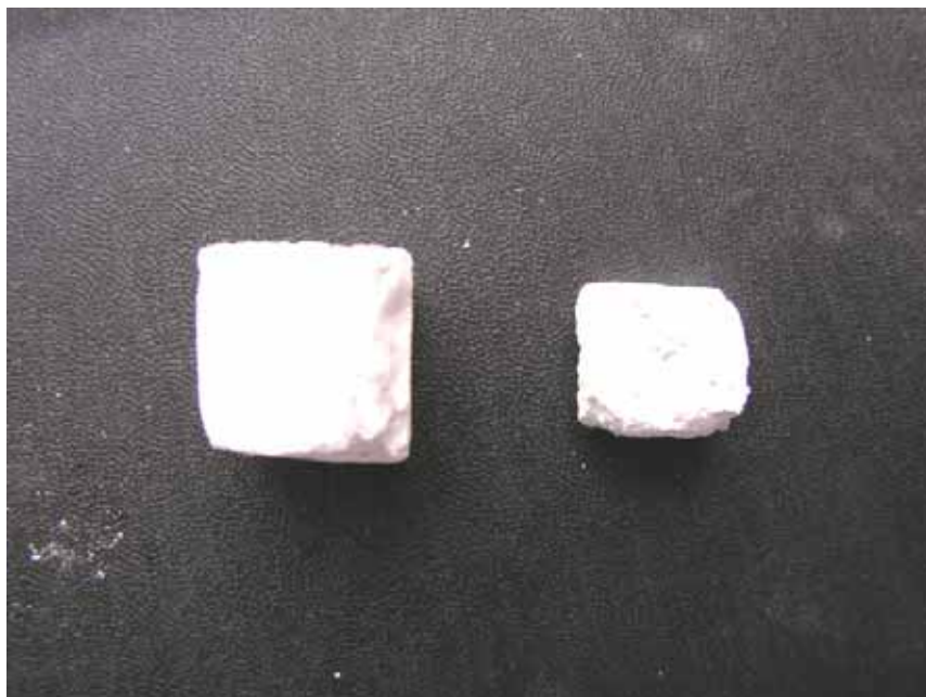
Fig. 2. Quartz ceramics, the samples of equal mass. On the left there is a composite obtained by synthesizing ceramics in a dispersion of carbon nanotubes, on the right there is a composite with carbon nanotubes grown in ceramic pores
