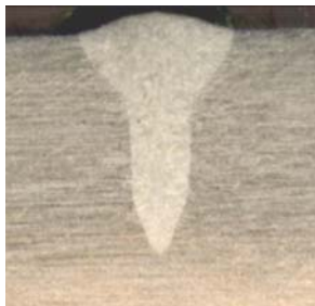
Fig. 13. Weld cross-section at 31 mA beam current, 826 mA no focus scanning, welding velocity 5 mm/s
