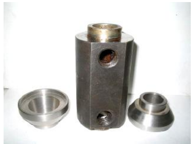
Fig. 1. Device for the study of viscous and plastic properties: a – scheme; b – the body of device with two adapters
