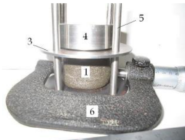
Fig. 3. Device and circuit measurement of Young's modulus and Poisson's ratio environment: 1 – sample of the working environment; 2 – base adjustment; 3 – weight bracket; 4 – extra weight; 5 – steered axles; 6 – micrometer
