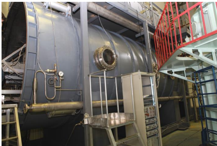
Fig. 11. The exterior of the GVU-60 test bench vacuum chamber
