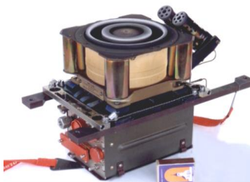
Fig. 1. Orbit raising thruster unit on the base of SPT-100B
