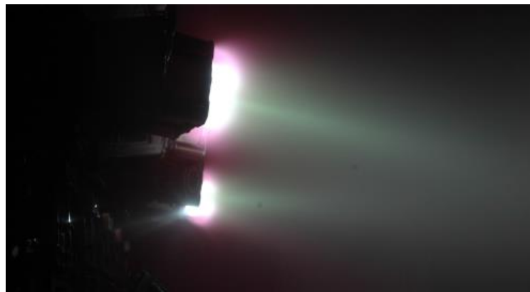
Fig. 13. Paired work of SPT-100B thrusters during the integration test
