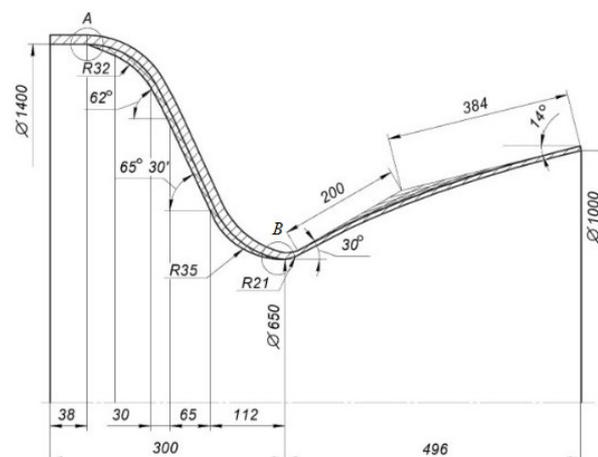
Fig. 2. SPRE nozzle with a CFRP (carbon fiber reinforced polymer) insert plate
