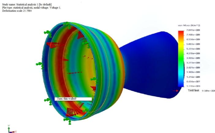
Fig. 5. Diagram of stress distribution in the nozzle  $t = 15$  mm
