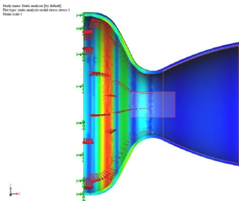
Fig. 10. Diagram of stress distribution in the nozzle  $t_{ti} = 20$  mm;  $t_{cm} = 7.5$  mm
