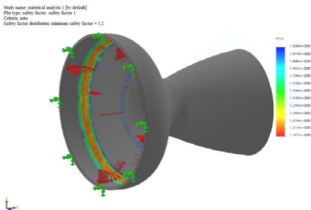
Fig. 7. Safety factor in the nozzle  $t = 15$  mm
