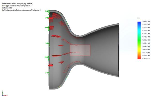
Fig. 12. Safety factor in the nozzle  $t_{ti} = 20$  mm;  $t_{cm} = 7.5$  mm
