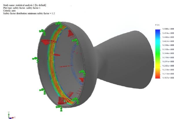
Fig. 8. Safety factor in the nozzle  $t = 30$  mm
