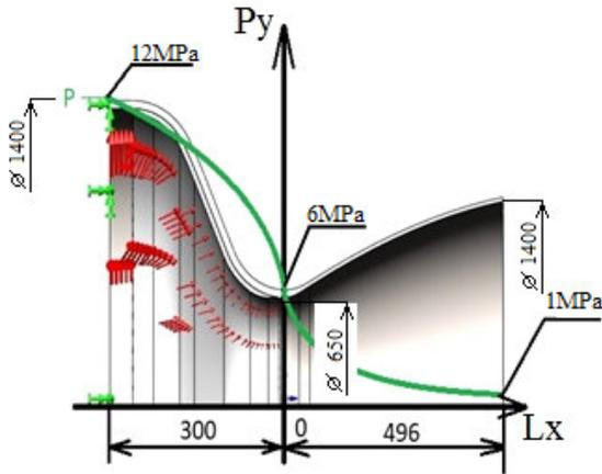
Fig. 3. Pressure distribution in the SPRE nozzle: P – pressure; L – length of the investigated zone
