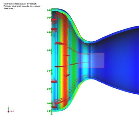
Fig. 11. Diagram of stress distribution in the nozzle  $t_{ti} = 20$  mm;  $t_{cm} = 17.5$  mm
