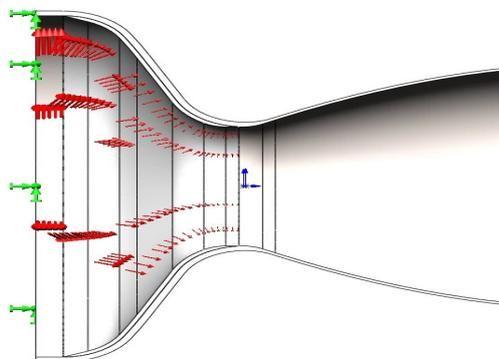
Fig. 4. Distribution of loads in the nozzle
