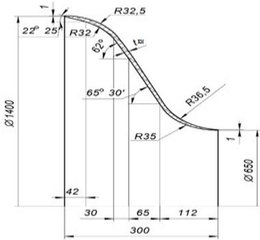
Fig. 9. Insert plate made of composite material
