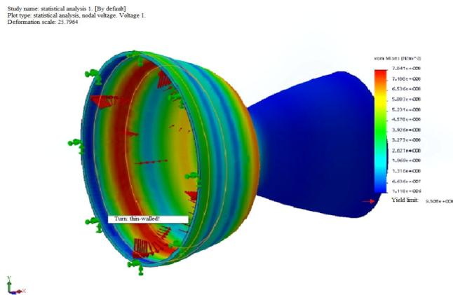
Fig. 6. Diagram of stress distribution in the nozzle  $t = 30$  mm
