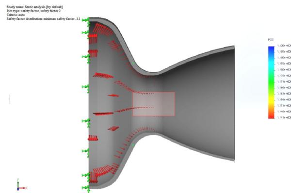
Fig. 13. Safety factor in the nozzle  $t_{ti} = 20$  mm;  $t_{cm} = 17.5$  mm
