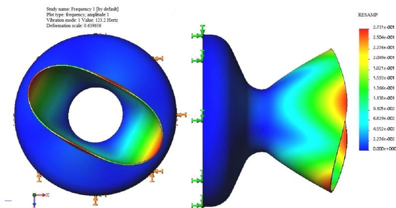
Fig. 14. Amplitude of the first mode of vibrations
