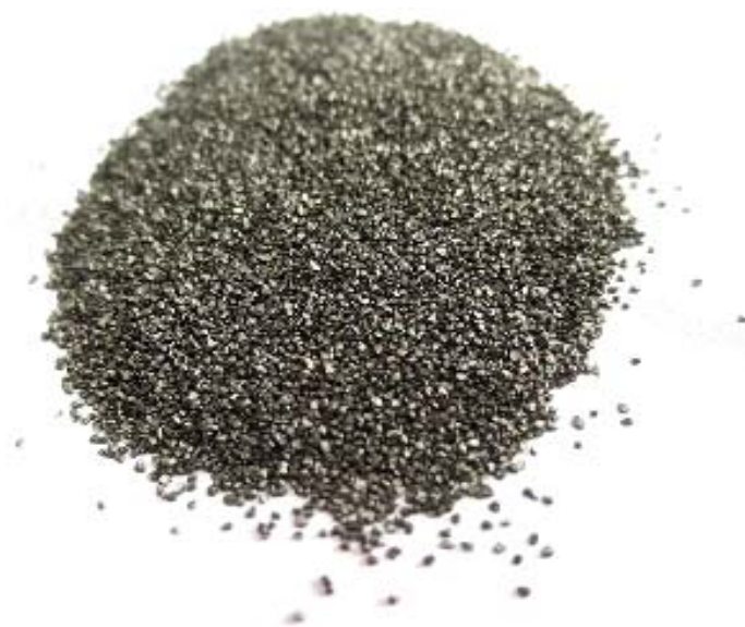
Fig. 2. The appearance of the dispersed filler modified with tungsten
