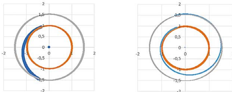
Fig. 1. SSS trajectory during Mars flyby and velocity compensation in Mars orbit
