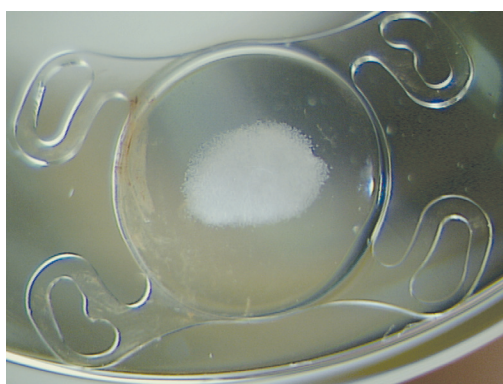
Fig. 2. Photo of an explanted intraocular lens with calcifications in the optical part
