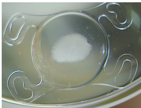
Fig. 2. Photo of an explanted intraocular lens with calcifications in the optical part
