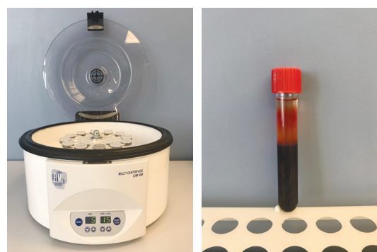
Fig. 2. Multi Centrifuge CM 6M centrifuge and laboratory test tube for producing platelet-rich autologous serum
