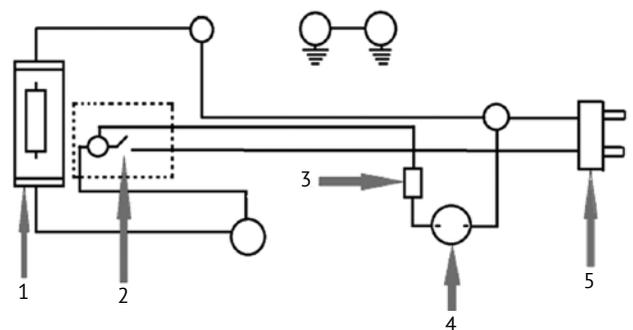
**Fig. 1. Circuit of the heating element for reproducing the thermal burn. 1, the heating element; 2, the thermostat; 3, the resistor; 4, the indicator lamp; 5, the main plug**
