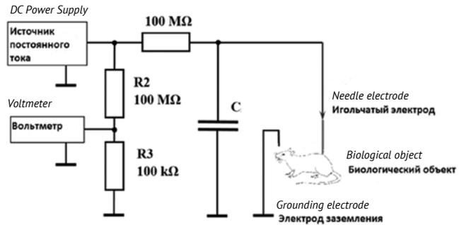
Fig. 3. Generator circuit of low-temperature low-pressure atmospheric plasma
