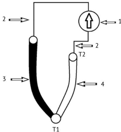
Fig. 2. Thermocouple circuit for high-temperature exposure dosage. 1, measuring device; 2, connecting wires; 3, 4, thermoelectrodes
