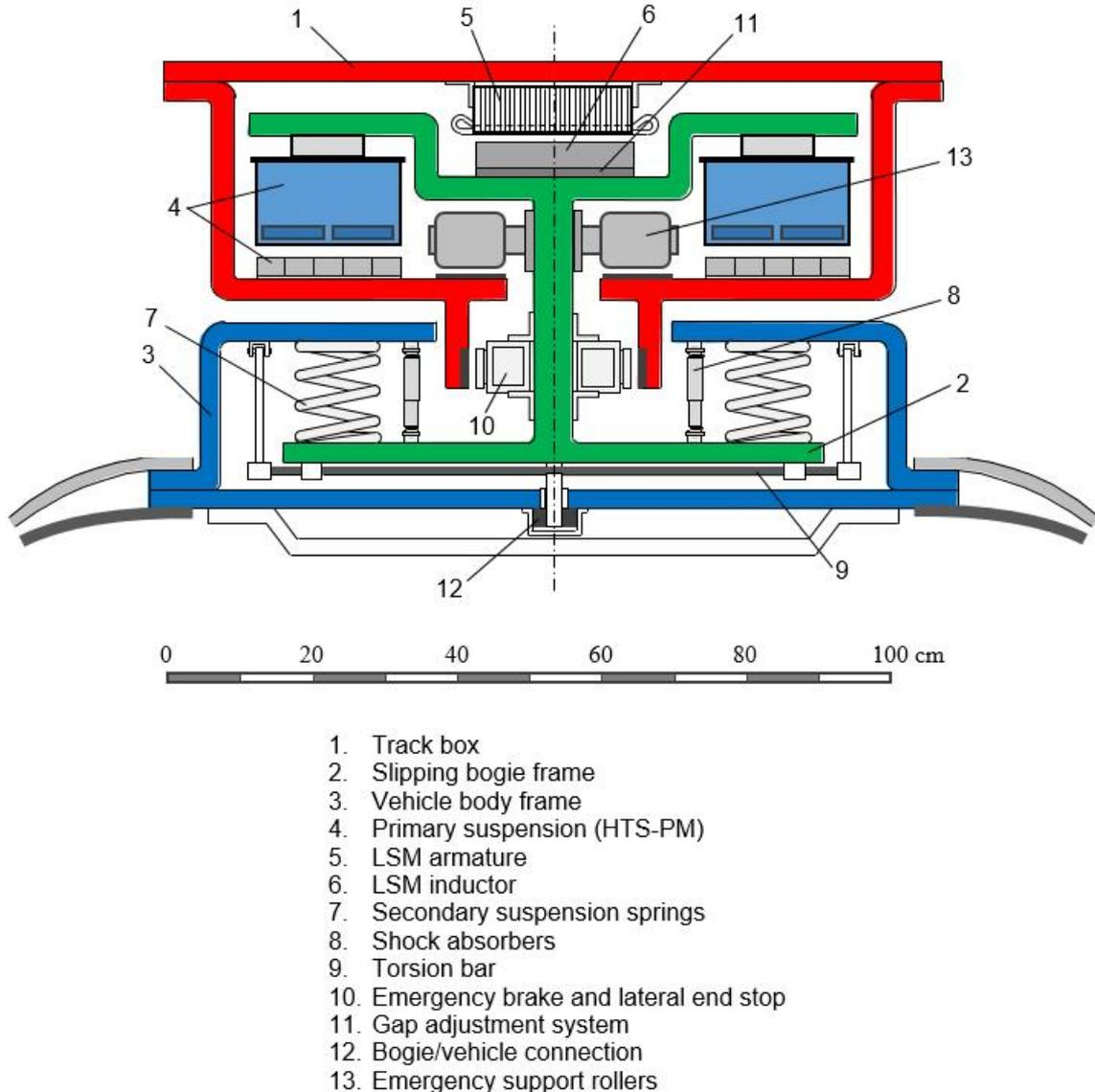
Fig. 6. The suspended Maglev system core – Solution B with HTS/PM primary suspension
