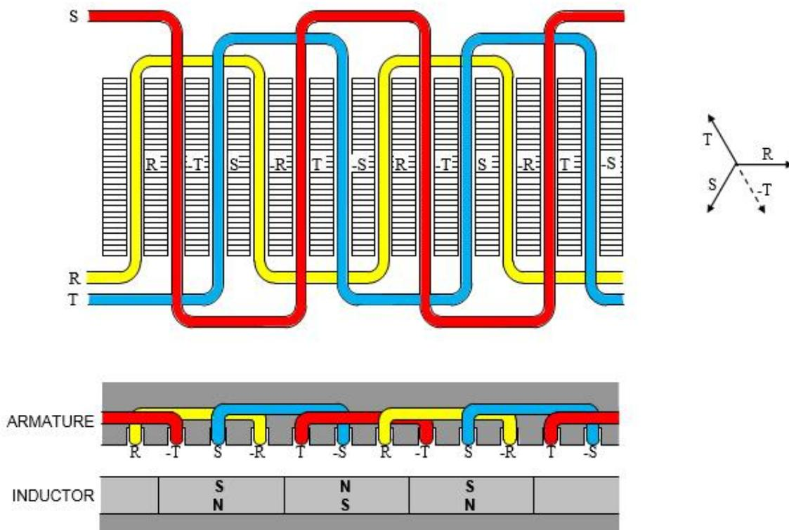
Fig. 7. The Linear Synchronous Motor (LSM)
