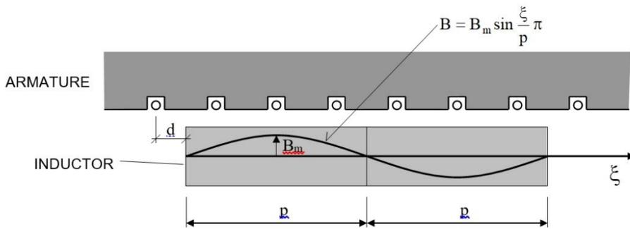
Fig. 9. Sinusoidal trend of induction within the inductor poles
