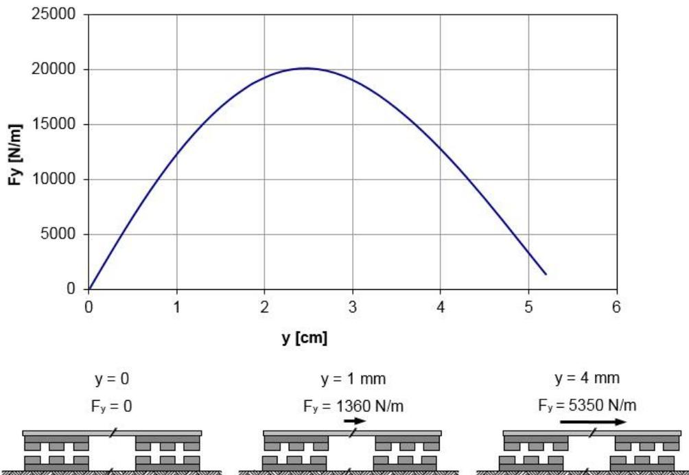
Fig. 5. Lateral force  $F_y$  as a function of displacement  $y$ , for magnets' composition of Fig. 3
