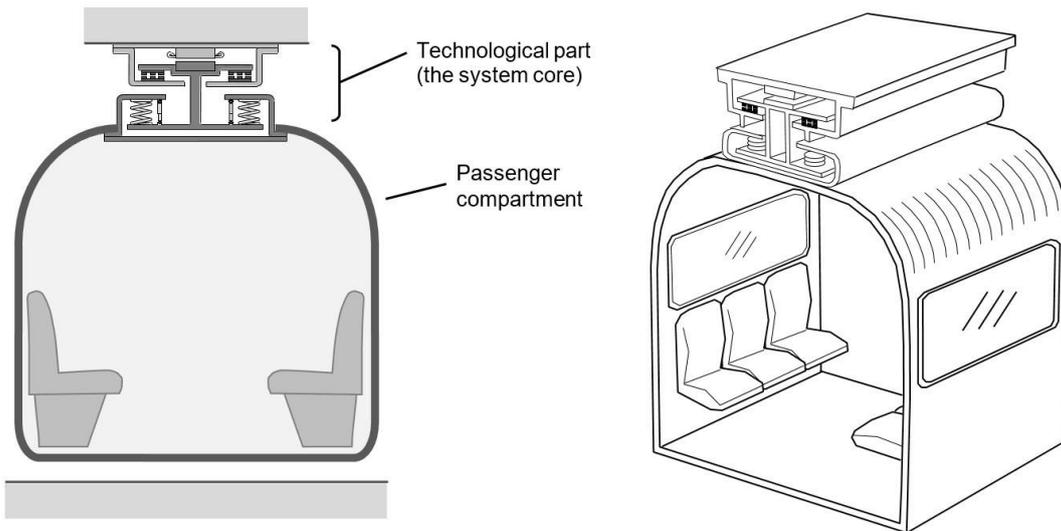
Fig. 1. The suspended Maglev configuration
