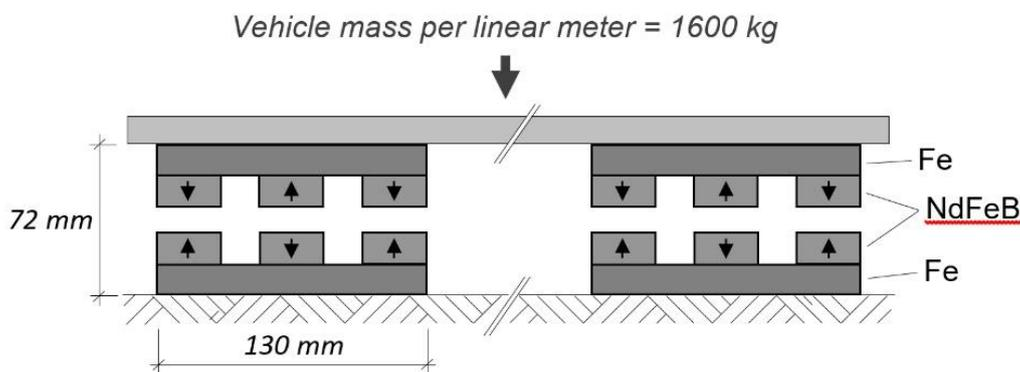
Fig. 4. Magnets' configuration to levitate a 1600 kg/m vehicle
