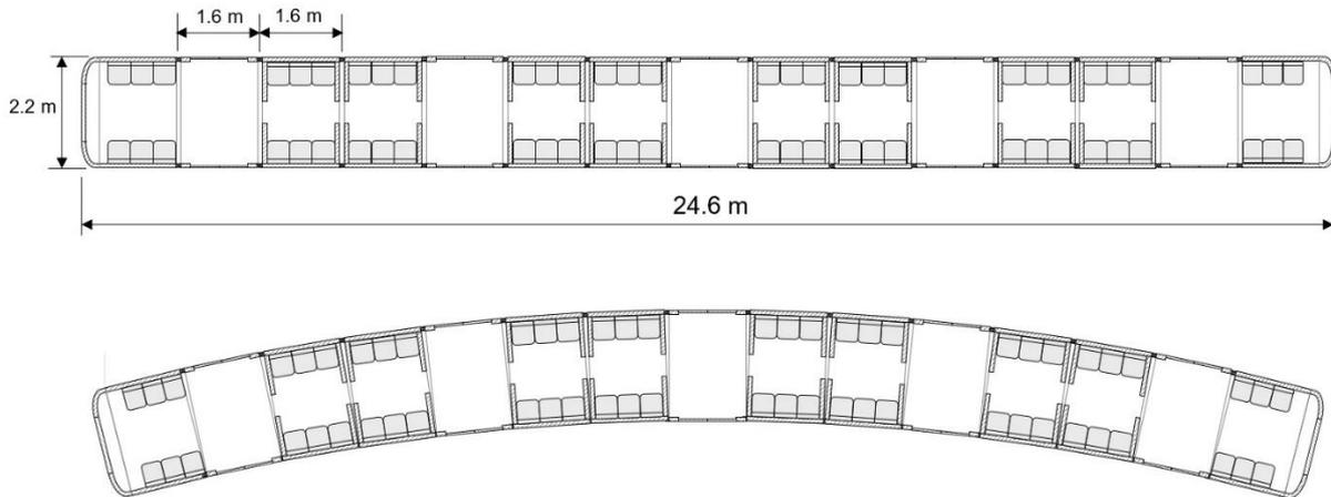
Fig. 3. Modular vehicle layout
