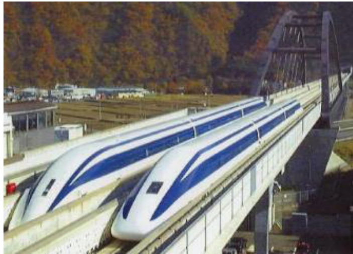
Fig. 14. EDS technology used in the JR-Maglev MLX01 Japanese System (Source: Central Japan Railway Company – Yamanashi Maglev Test Line, 2000)
