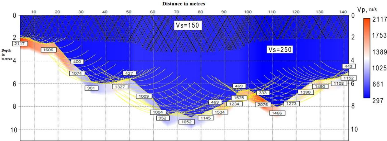
Pic. 2. Generalised velocity profile I. Hatched lines – lower boundary of subgrade, detected by virtue of MASW
