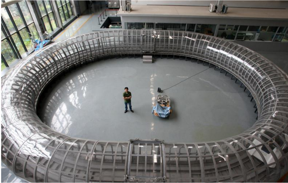
Fig. 25. Test facilities of the evacuated tube HTS maglev train
