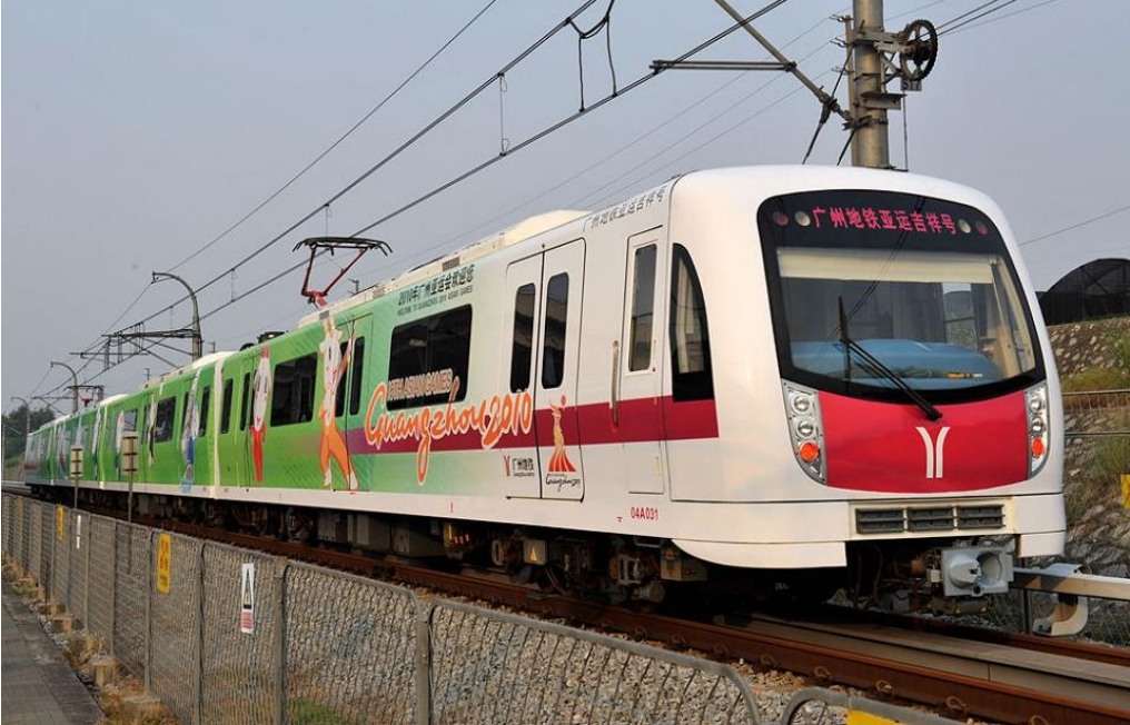
Fig. 15. Linear train in Guangzhou metro line 4
