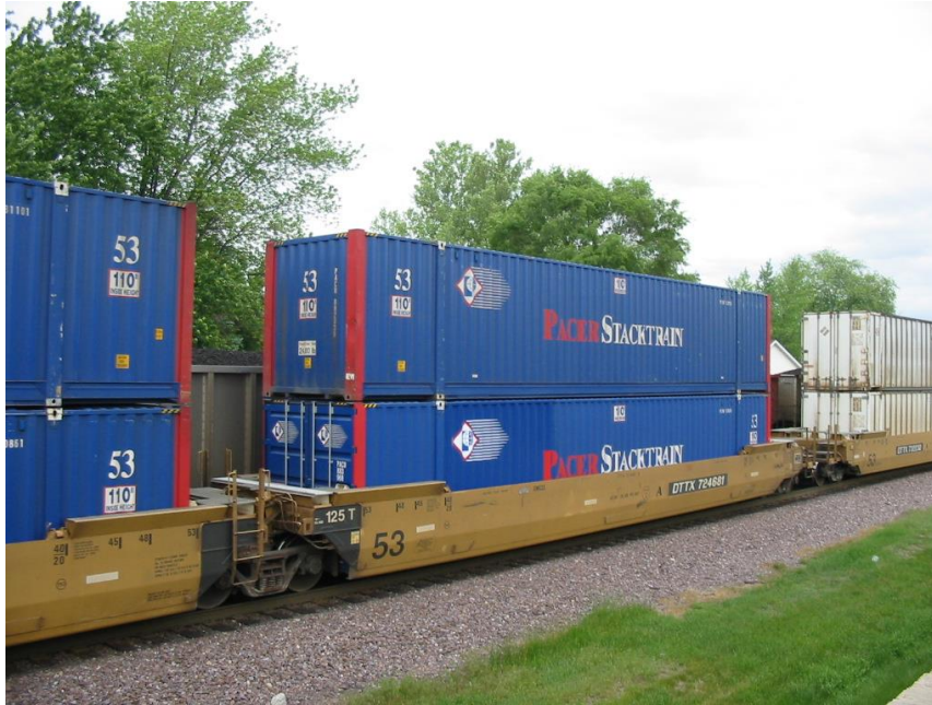
Fig. 2. Double-stack transportation on the platform with the depressed floor on the USA railways
