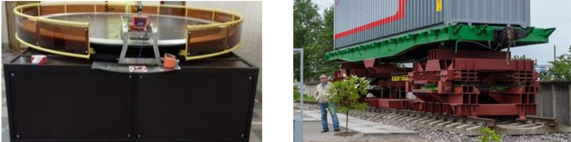
Fig. 5. A laboratory stand (a) and a test model (b) for research of the magnetic levitation transport technologies
