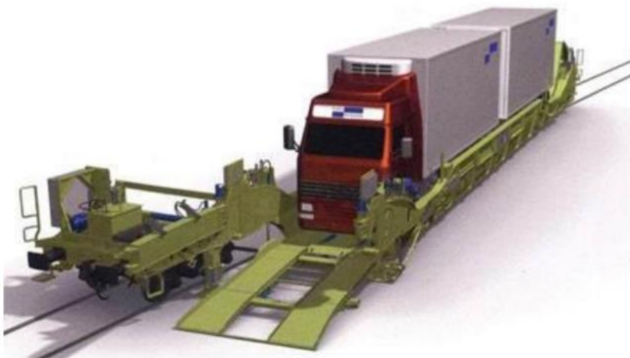
Fig. 8. Swing-deck of the system Flexiwaggon
