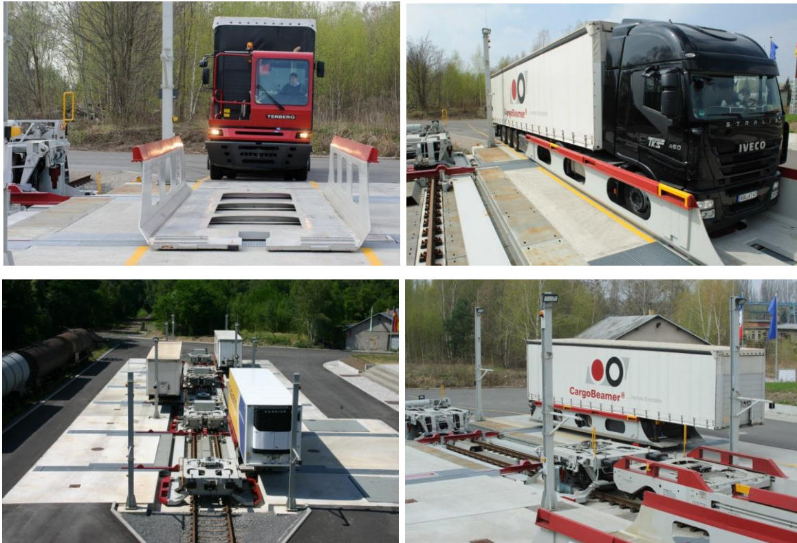
Fig. 14. The technology scheme of the loading of the trailer on the the CargoBeamer platform
