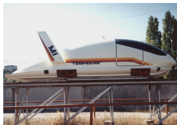
(e) Test track of aero-electrodynamic suspension of the vehicle (Dnepropetrovsk city, Ukraine)
