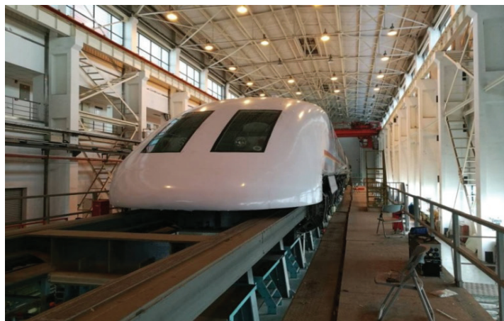
Fig. 9. The high-speed maglev train based on hybrid permanent magnet and electromagnet in Shanghai
