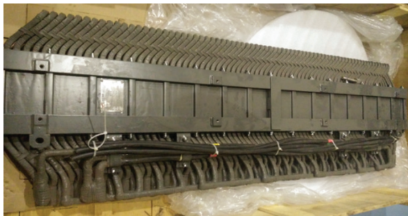
Fig. 7. The Original LIM (1820 mm)
