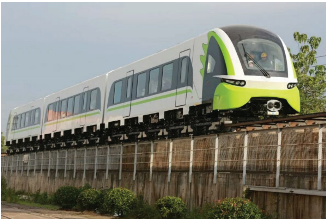
Fig. 7. Version 2.0 commercial maglev train with speed grade of 160 km/h
