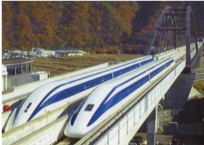
Fig. 14. EDS technology used in the JR-Maglev MLX01 Japanese System
