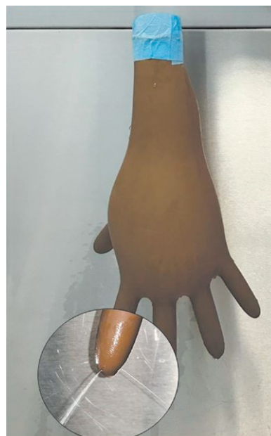
Fig. 1. Method of investigation of damage to surgical gloves
