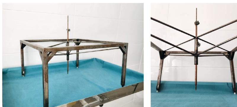
**Fig. 3.** Photographs of the impact rig in the assembly
